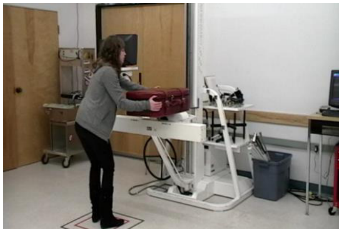
Fig. 1. Participant standing in a marked area in front of the target suitcase (54.57 L) mounted on the LMD of the LIDO WorkSET.
