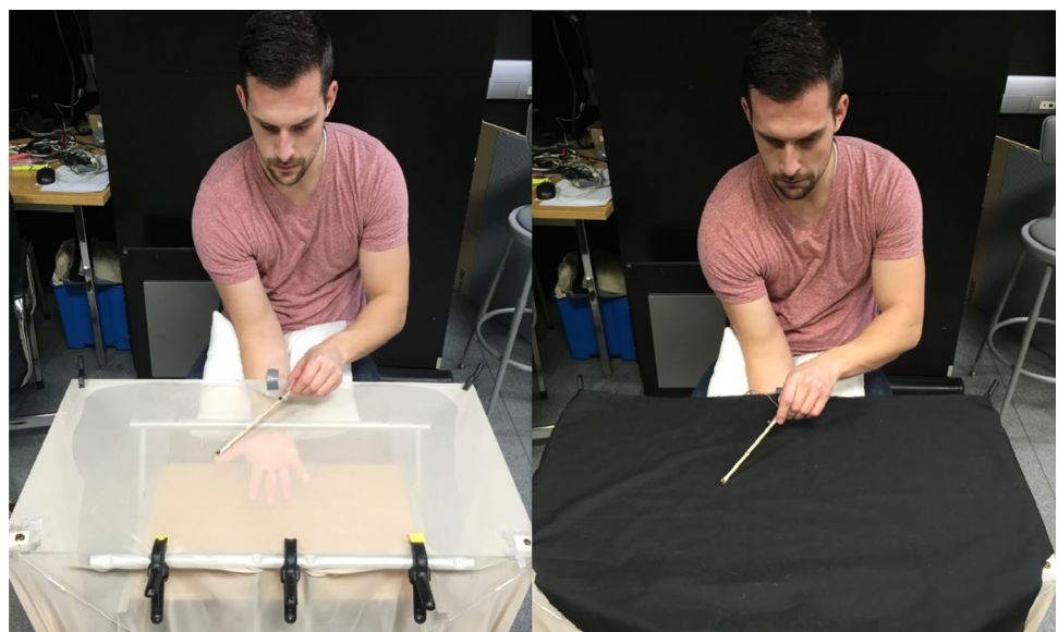
Fig. 1 This was the experimental setup for the experiment. The participants sat with their hand pressed up against the glass tabletop. They pointed using the wooden stylus. The black table cloth restricted vision of the participant’s hand in the occluded trials
